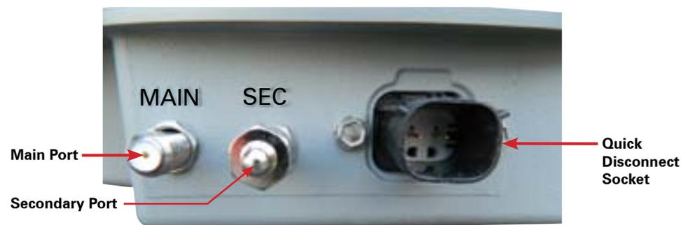
Connect coax to the main connection on the base of the antenna. Do not use a wrench to tighten the cable. The coax provided uses weatherproof connectors, which can be damaged if over-tightened.
