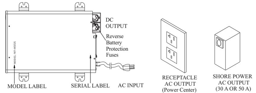
If the reverse polarity fuses are blown, it means the RV battery was accidentally connected in reverse, either at the battery or at the converter. Reconnect properly, then replace the fuse with the same type and amp rating as the original “Littelfuse®” Type 257 automotive-style fuse.
