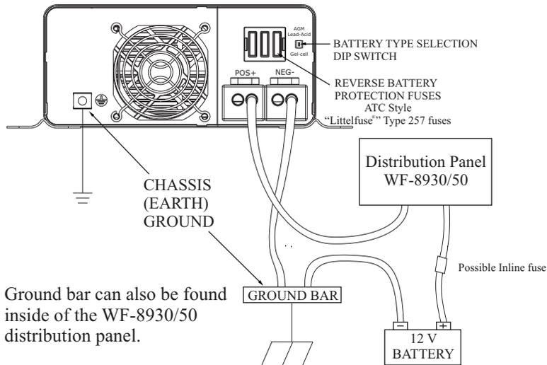
If the converter output voltage reads in the 13.2 Vdc-14.4 Vdc range and the battery is not charging, check for:
