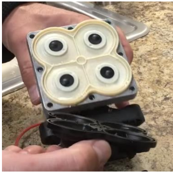
Figure 6. Remove the diaphragms (the black portion in this photo).
