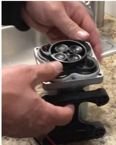
Figure 8. Place the diaphragms onto the pump.
