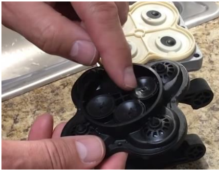
Figure 7. Check the diaphragms for debris.
