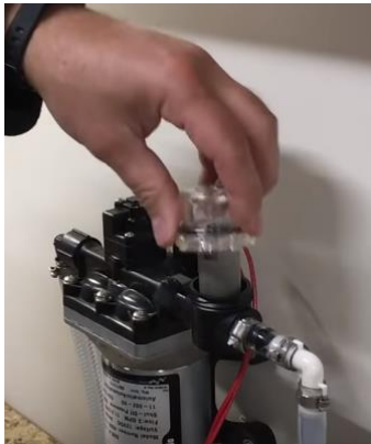
Figure 2. Removing or installing the clear cap.
