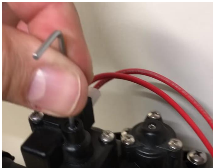
Figure 4. The 5/64 allen wrench (allen key) adjustment point.
