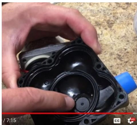
Figure 5. The check valve.
