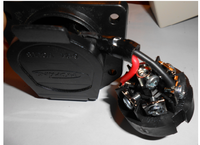
Inside of Bargman 7 pin - vehicle side
