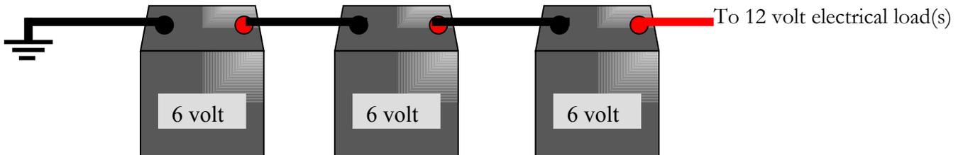
**NOT LIKE THIS!** Adding a third battery in series with the other two would give us the same 100Ah, but at **18 volts**, and 18 volts would burn out every 12-volt light bulb, motor, and battery operated appliance in your RV! Don't do it. What you need is not a series connection or a parallel connection, but a *combination of the two*, shown next.
