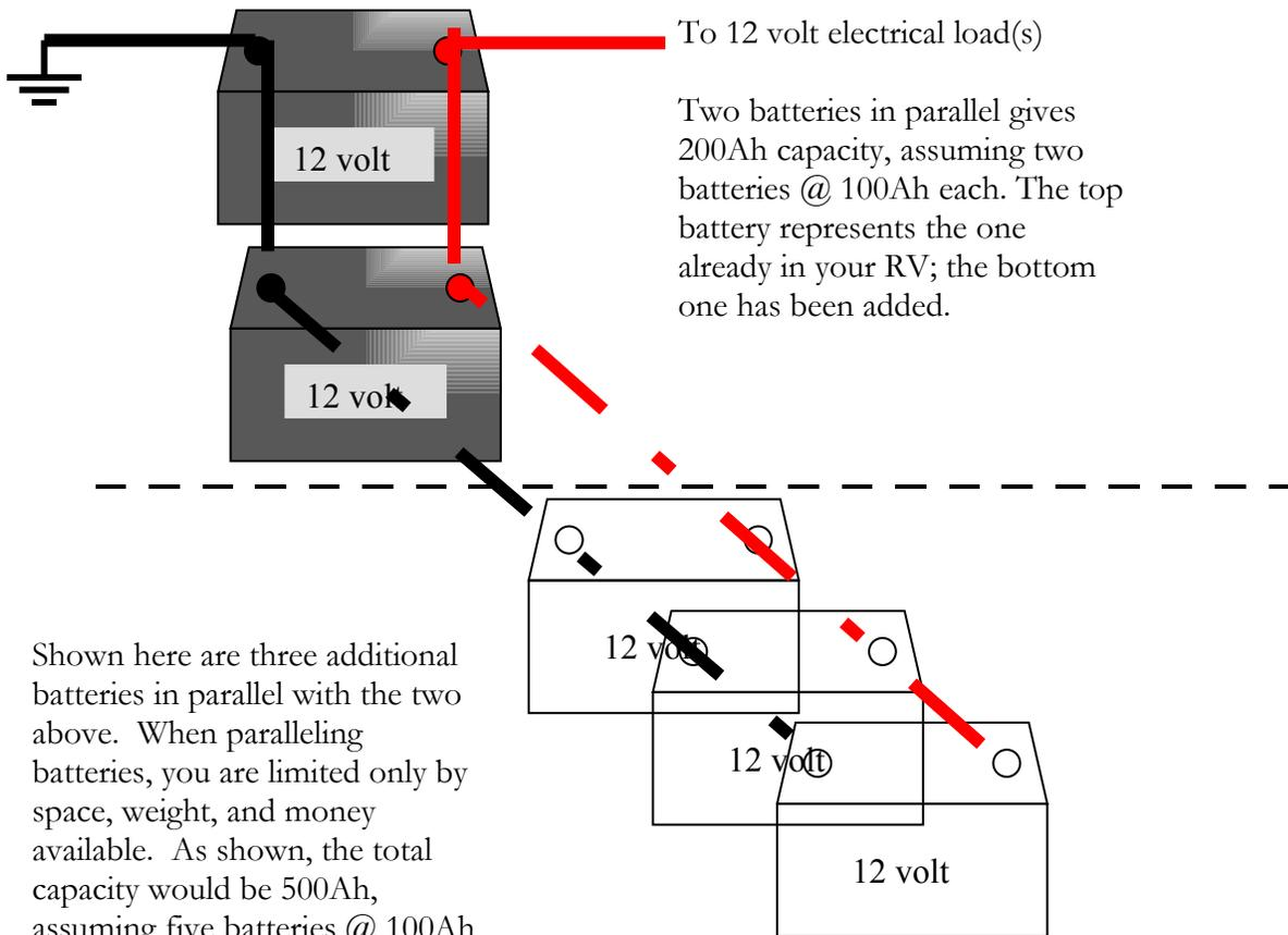
Shown here are three additional batteries in parallel with the two above. When paralleling batteries, you are limited only by space, weight, and money available. As shown, the total capacity would be 500Ah, assuming five batteries @ 100Ah each.
