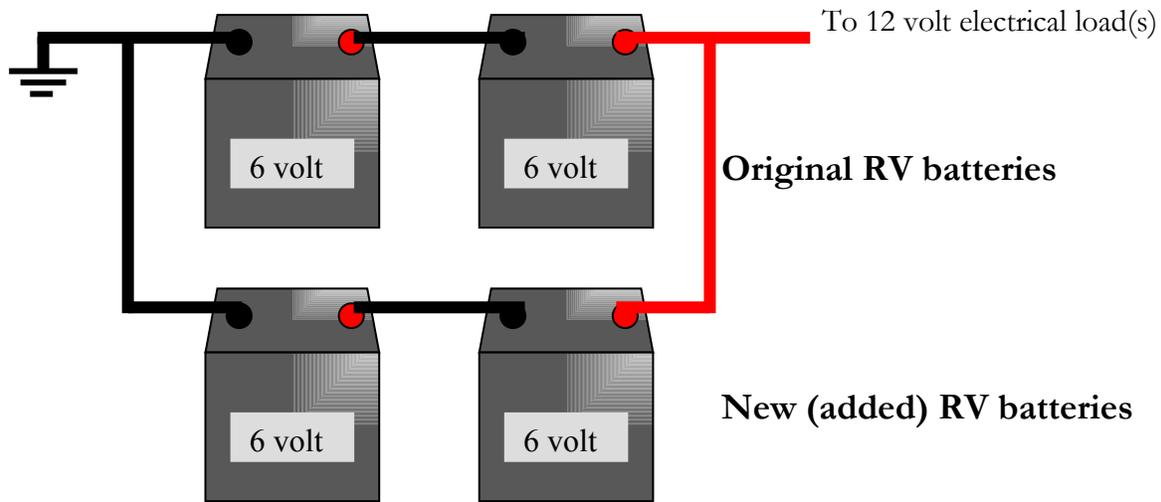
This is what we get. Because we added the two new batteries in parallel to the existing two batteries, we have doubled our Ah capacity from 100 to 200, yet kept the voltage at 12 volts. Pretty neat, isn't it?
