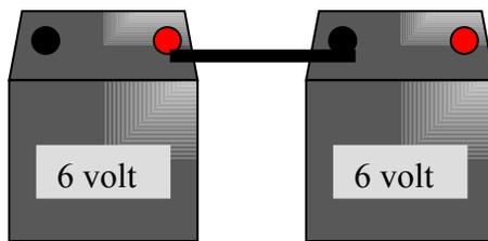
As you can see, they too are in series (positive terminal of one battery to the negative terminal of the other), but they don't connect to anything yet. Let's do that now, just as we did when we hooked up two 12-volt batteries in parallel.
