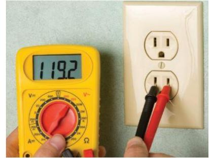
The meter setting will need to be changed to **AC volts** which may be indicated by **V~**. The range will need to be set to **200** if the meter has range selections. After setting the meter, push the lead tips into the outlet and take your measurement.
