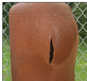
Fire damage, cracks and bulging
