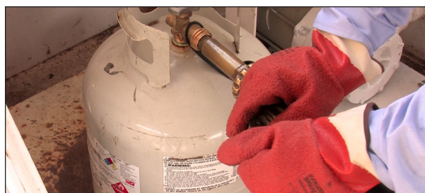
Operator closing hose end valve
