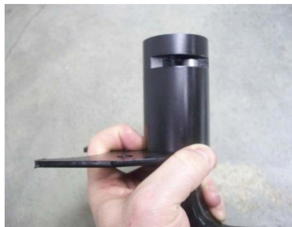
**Step 6:** With the tail end of the Spring Bar facing the trailer, insert the Spring Bar Bushing back into the bottom of the Main Hitch Head and replace the 3/8 bolt and lock nut. Tighten the lock nut firmly.
