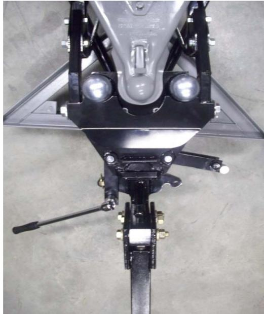
**Step 3:** Grease the hitch ball with all-purpose grease.
