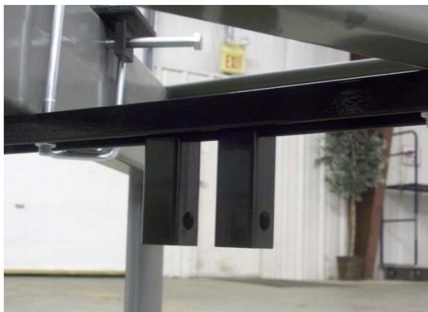
**Step 7:** Tighten the U-Bolt Hex nuts with your 11/16" socket.
