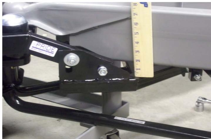
**Step 11:** Tighten the side Yoke bolts shown in the picture above.
