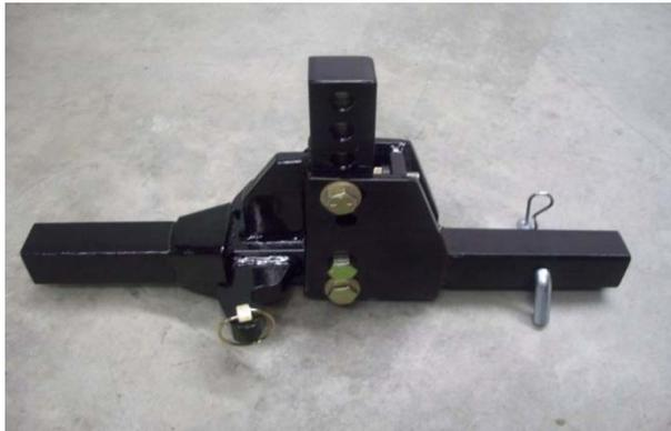
**Hitch Bar Assembled Plates DOWN – Offset between Tow Vehicle number and Hitch Box number.**
