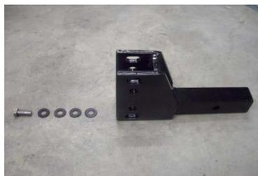
**Step 6:** Hitch Bar Hitch End assembly. If you used 4A or 4B above your Hitch Bar Hitch End will be like shown in the parts picture above with the adjustment holes facing UP. If you used 4C or 4D above your Hitch Bar Hitch End will have the holes facing DOWN.
