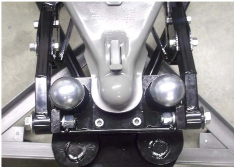
**Step 5:** Tighten the 3/4" Bolts VERY TIGHT. These bolts MUST BE TIGHT. Torque to 250 ft-lbs. Repeat on both sides of Yoke.
