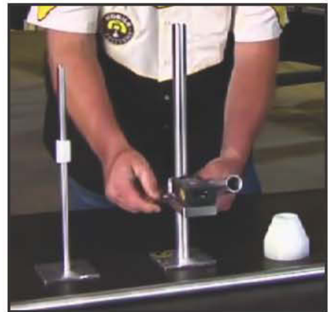
2. Install laser alignment tool.
