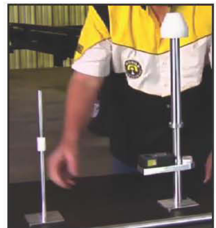
5. Install Kingpin adapter (Fits 2" - 2 1/2" Couplers).
