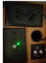
Power Injector Green Light = ON
