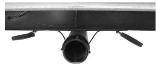
Black/Grey tank drain & valves
