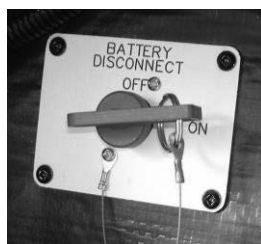
Battery Disconnect Switches
