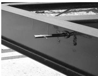
Fig. 1-Through Frame Crank Extension w/ pin
