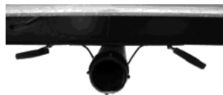
Fig 8.8 Black/Grey tank dump valves
