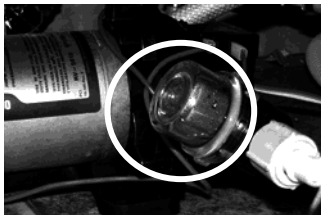
Fig. 8.3 Water pump strainer
