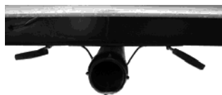
Fig 8.8 Black/Grey tank dump valves
