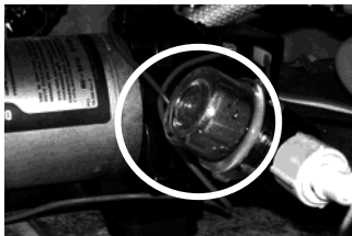
Fig. 8.3 Water pump strainer
