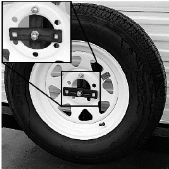
Fig. 4.4 Spare tire carrier installation
