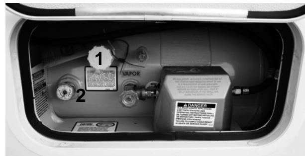
1: Propane fill valve; 2: Propane gauge
