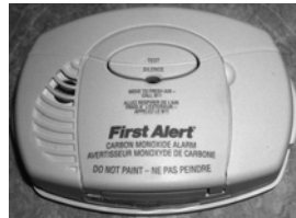
Fig. 2.4 Typical CO alarm
