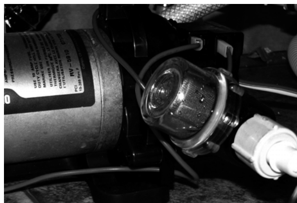
Fig. 7.3 Water pump strainer
