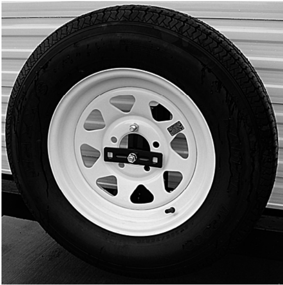
Fig. 5.2 Spare tire carrier installation
