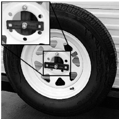
Fig 5.2 Spare tire carrier installation
