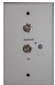
Fig. 11.3 TV Power Supply
